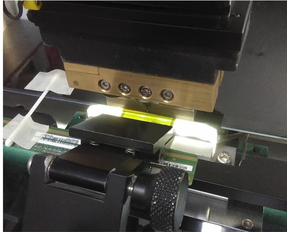
When bonding finished, can check the bonding effect with the screen, each pin on Glass and COF should connect in a good quality. If not connect very well, please disassembly the COF and re-bond it carefully.
