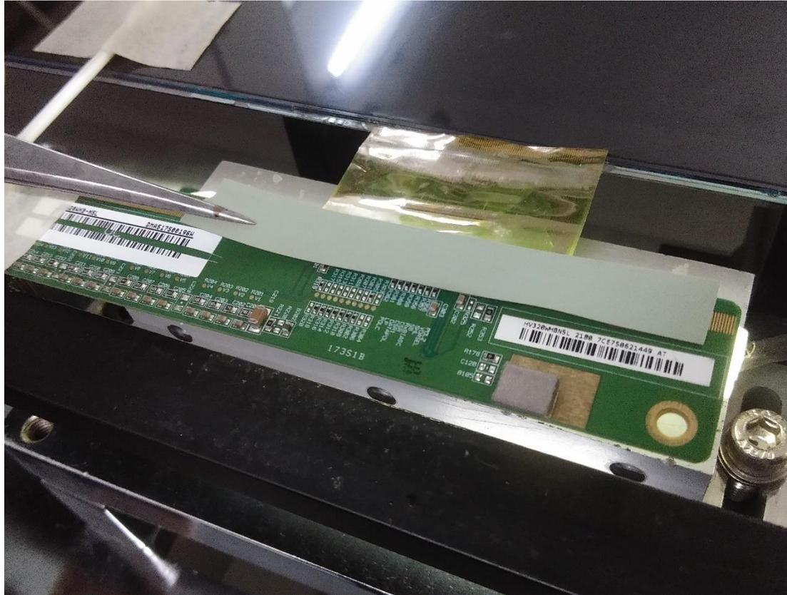
After alignment, put a silicone table on the COF, it will protect the COF and make the heating more uniform. Please note, ITO side use Teflon and PCB side use silicone. The length of silicone tape should longer than COF length.
