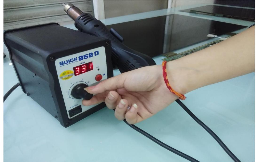
A properly parameter of the hot gun can make the COF flat, non-deformation, and unshrinking during removing.
