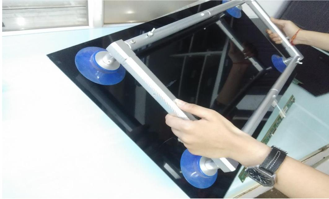
After cleaning, move the ITO to bonding machine platform by two hands. Please note should put two hands in the center of the ITO. Make sure the ITO is smooth and steady.
