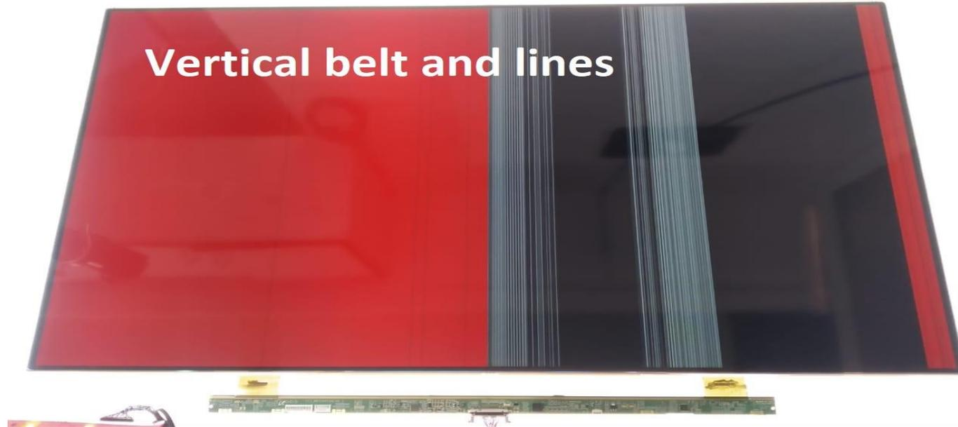
Make a mark on the screen where fault appear (Vertical line, belt; Horizontal line, belt), after bonding check again if the fault disappeared.
