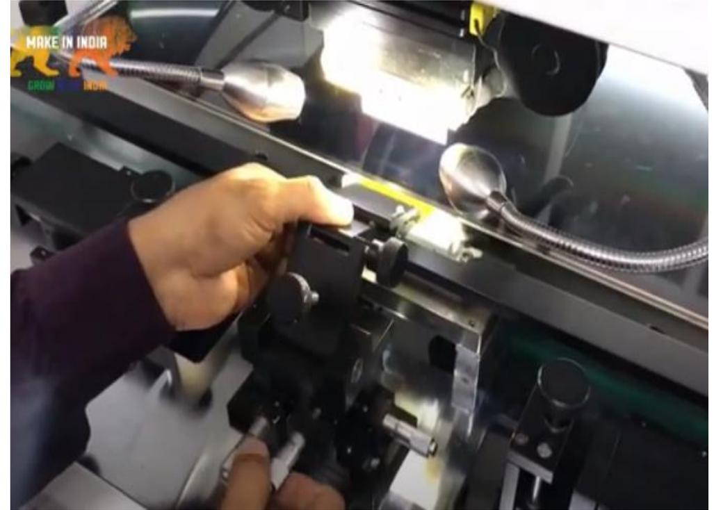
Open the COF fixture, put the COF in fixture, the fixture should not touch the chip on COF. Remove the protection film of ACF. Then put the COF on glass pins and align them.
